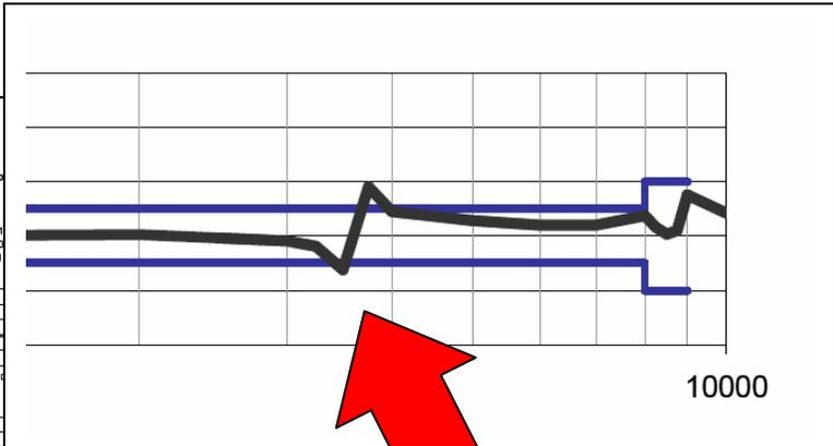
Figure 8. Calibration certificate from the 0° angular position, amplitude response exhibiting large glitch near 3500 Hz exciter resonance
