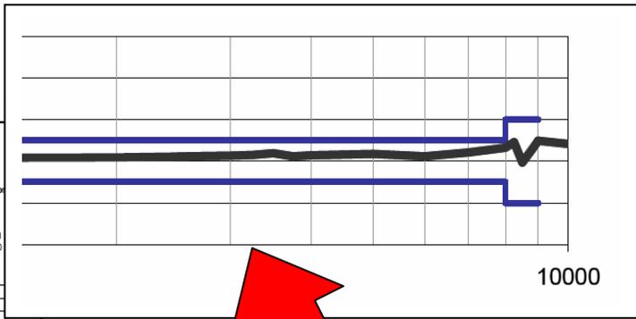
Figure 7. Calibration certificate from the 90° angular position, amplitude response exhibiting small glitch near 3500 Hz exciter resonance
