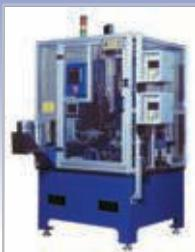
Eddy Current Cylinder Liner Testing System
