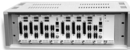
**Figure 3** - Computer Controlled Signal Conditioning System Powers 96 Transducers (Bank Switching Into 32 Data Acquisition Channels) In A 19-Inch Rack Mount.
