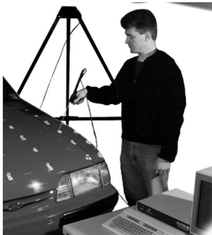
**Figure 6** - 3D Sonic Digitizing Automates The Structure Geometry Definition Process
