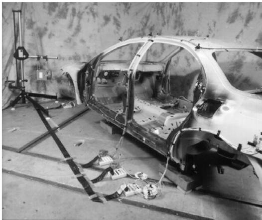
**Figure 2** - Shielded Multi-conductor Ribbon Cables Gather Transducer Signals At a Central "Hub", With Single Channel "Spokes" Extending Over The Test Structure.
