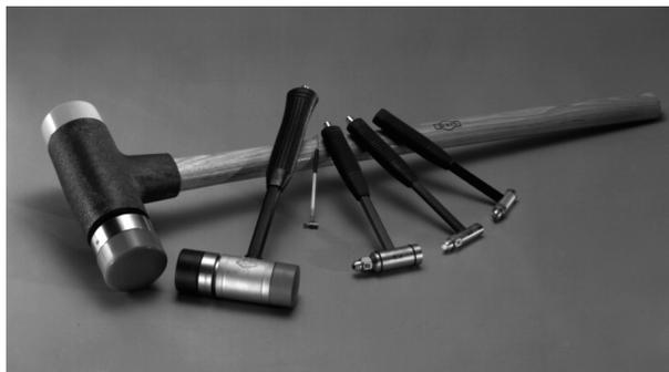
**Figure 2-2.** Collection of Hand-Held Impact Hammers.
