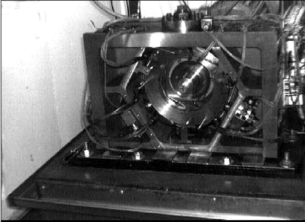
**Figure 4-27.** Squeeze Film Damper Rig Test Case.
