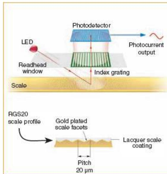
Figure 7. Optical Encoder Operation (graphic courtesy Renishaw)
