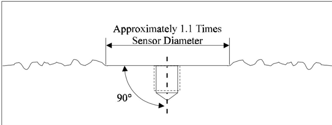
Figure 1: Mounting Surface Preparation
