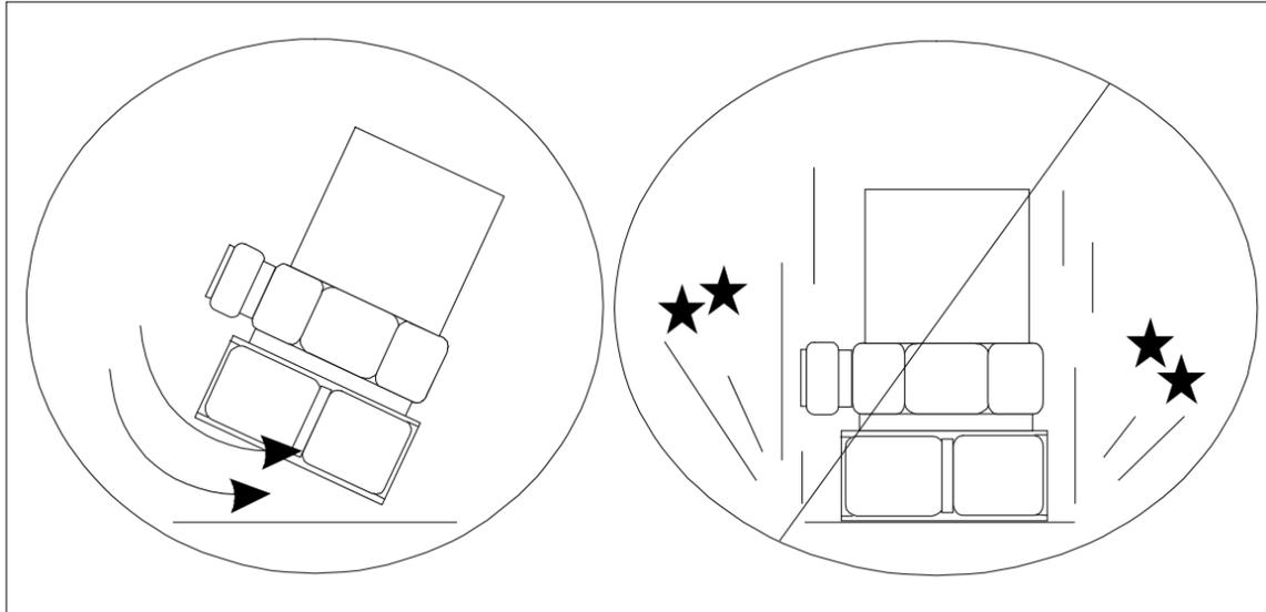
Figure 5: Magnet Mounting
