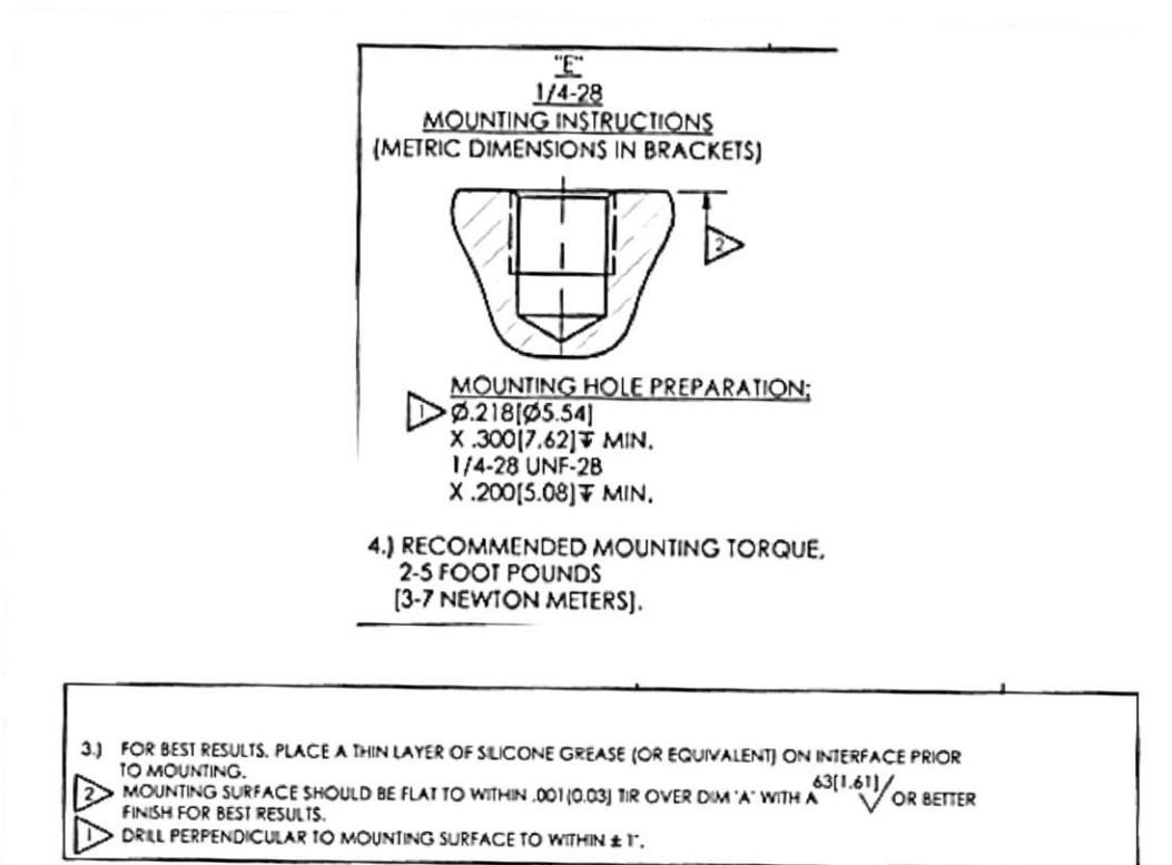
Figure 2: Mounting Surface Installation Drawing
