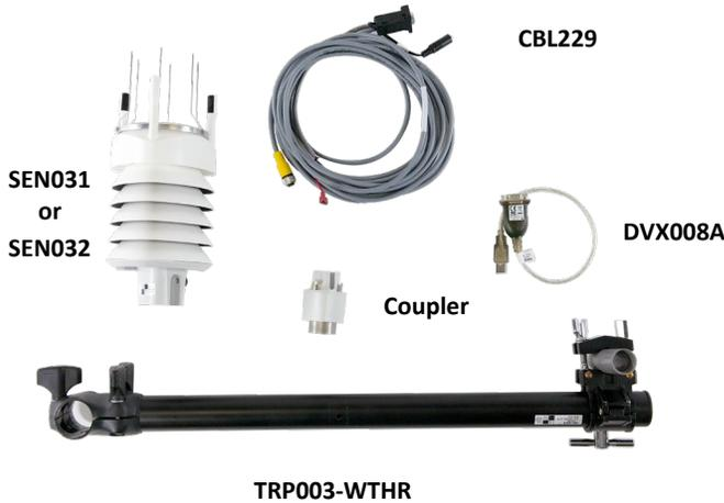
\_\_\_\_\_ **SEN031** Combined weather sensor: wind speed and direction, temperature, humidity, pressure, rainfall (includes coupler)
